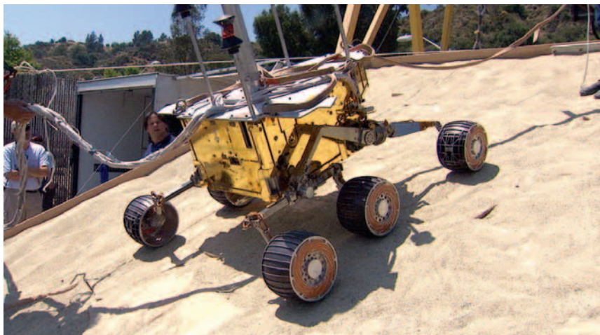
A rover test drives up a manmade slope at JPL to simulate conditions it will face in "Endurance Crater." The test rover successfully descended and climbed the platform, adding confidence that Opportunity could cross a similar hurdle in Endurance Crater. Image credit: NASA/JPL
