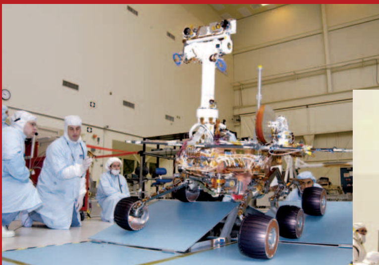
Above: Rover 2 is driven over staggered ramps to test the suspension’s range of motion.
